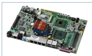
3. Intel mobile technology supports multiple processors from Fanless ULV CPU to high performance Celerm M, Core 2 Duo.
